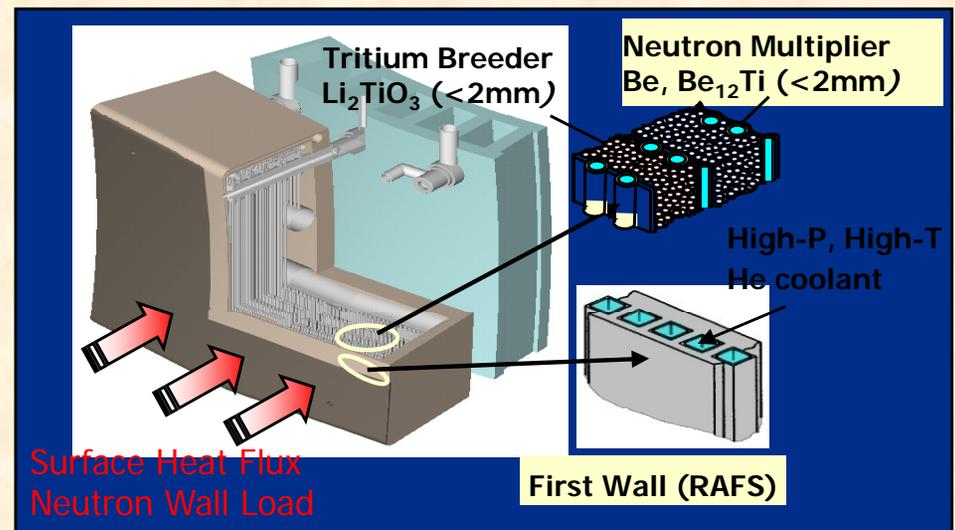
↑ *Blanket example: Typical vision of a ceramic-breeder-based blanket module.*
