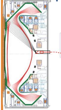
Imaging spectrometer for standard and advanced divertor configuration studies (strike points, X-point)
