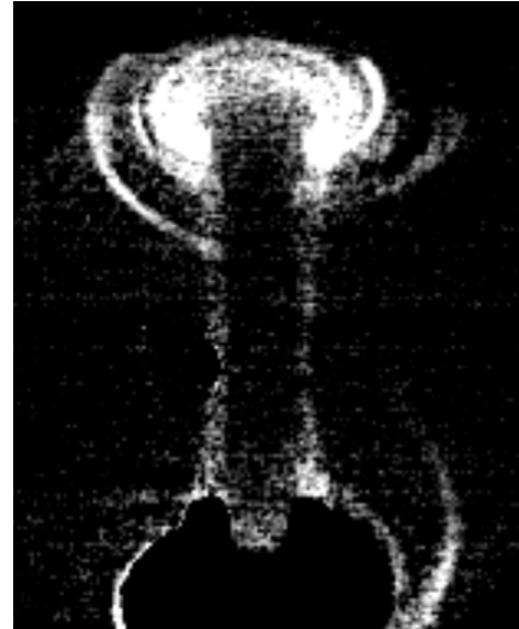
Fig. 5.2.1.3- filamentary structure of Type V ELM on wide angle camera.
