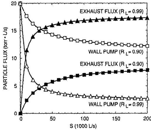
Fig. 4. Divertor exhaust and wall pumping as a function of recycling and pumping speed.
