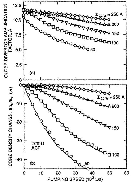
Fig. 6. (a) Outer divertor amplification factor (ratio of divertor particle flux to throat particle flux)  $A \sim 9\text{--}12$  for  $\Sigma_{\text{core}} \sim 150\text{--}250$  A. (b) Predicted core density change with pumping. Large decreases are predicted with low core fueling rates. The PREVORTEX model predicts particle confinement times from 150 to 300 ms, with an assumed ELM diffusivity of  $10^4$  cm<sup>2</sup>/s.
