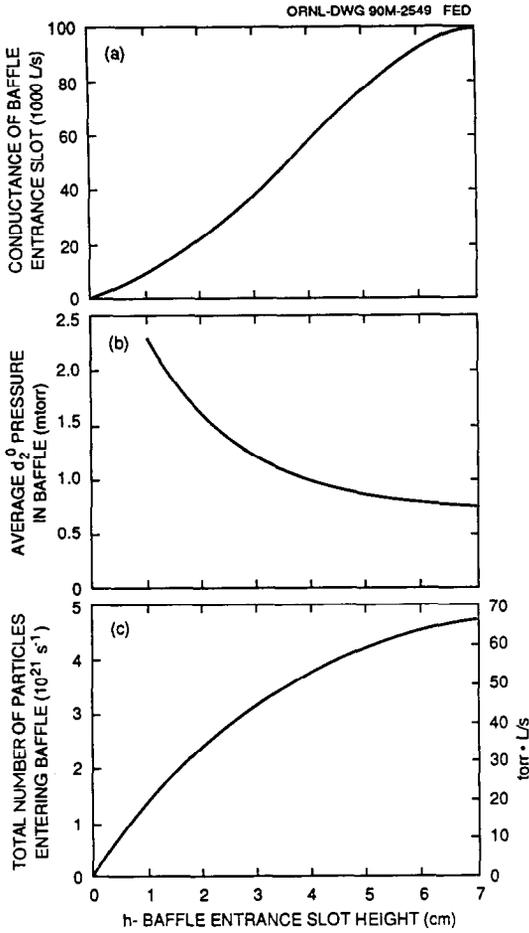
Fig. 2. (a) Conductance of baffle entrance slot, (b) average  $D_2^0$  pressure in baffle, and (c) total number of particles entering baffle as functions of baffle entrance slot height.
