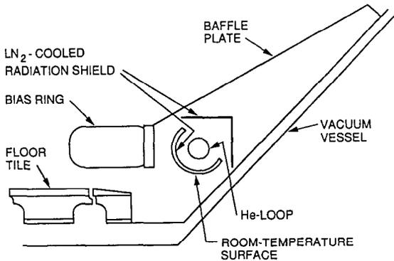
Fig. 3. Configuration of the baffle, bias ring, and cryopump system optimized for  $S = 50000$  L/s. Approximately 50% of the neutral flux into the baffle is pumped.
