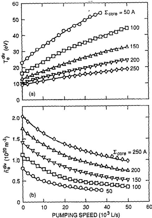
Fig. 5. Variation of (a) the outer divertor plate temperature and (b) the electron density at the outer divertor plate as a function of pumping speed for central fueling rates from 50 to 250 A. Temperatures in the range from 10 to 20 eV are predicted for  $\Sigma_{\text{core}} \sim 150\text{--}250$  A (1 A =  $6.25 \times 10^{18}$  particles/s = 0.09 Torr · L/s).
