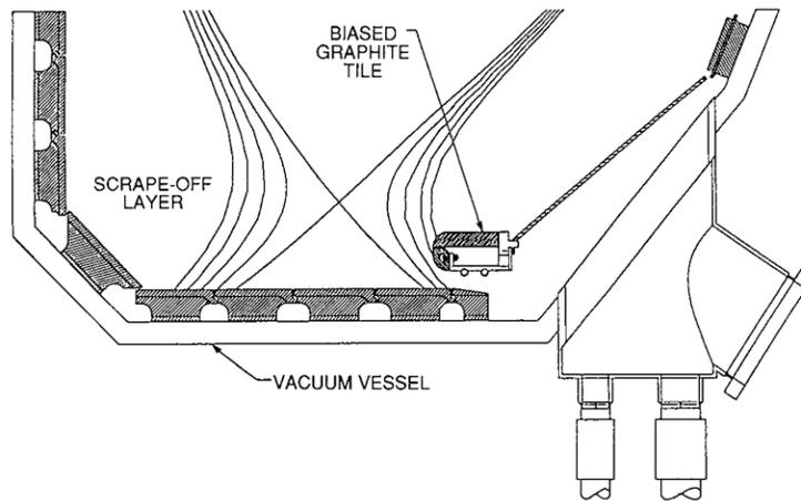
Fig. 1. Schematic view of divertor baffle and scrape-off layer near the strike points.
