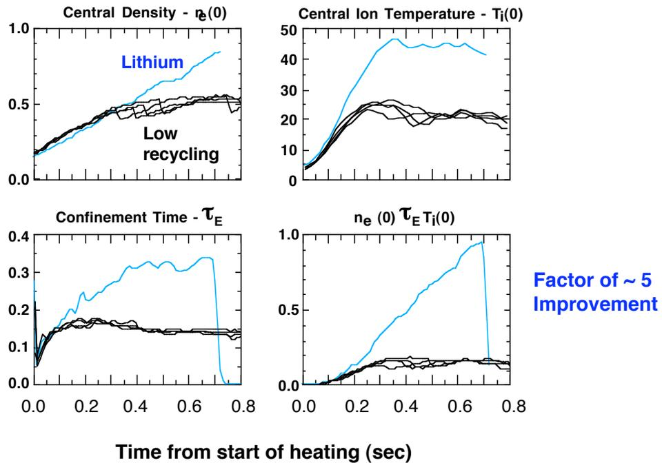
The impact of lithium wall coating on TFTR plasma performance was dramatic. Core confinement was substantially improved; central temperature and density increased as lithium further reduced recycling compared with well-conditioned, already low-recycling walls.
