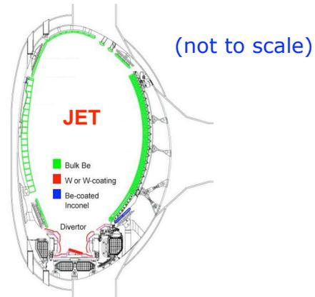
**ITER's low temperature Be first wall does not extrapolate to CTF/FDF or Demo.**
