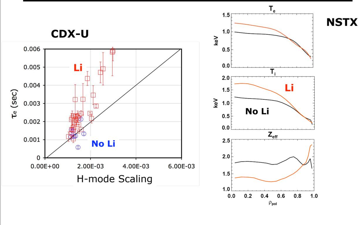
CDX-U has seen dramatic pumping with liquid lithium, and achieved approximately 2x H-mode confinement in Ohmically heating plasmas with lithium coating, as measured with magnetic diagnostics. NSTX has also seen significant improvement in performance with lithium evaporation in the divertor region.
