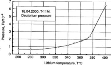
Results from T11-M (PP&CF **44**, 955) showing deuterium desorption vs. capillary lithium limiter temperature
