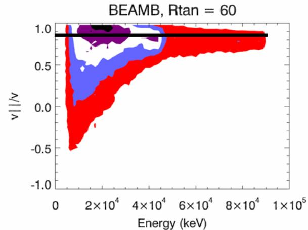
Average Pitch of Beam Particles in NPA sightline
