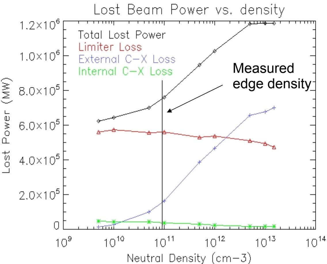
TRANSP calculations show the loss of beam power due to interaction with the edge neutrals. The increase in power lost by external charge exchange leads to a significant increase in the overall loss of beam power. At the edge neutral density measured by the ENDD ( $1-1.5 \times 10^{11}$ ), the total lost power is about 10% of the total input power.
