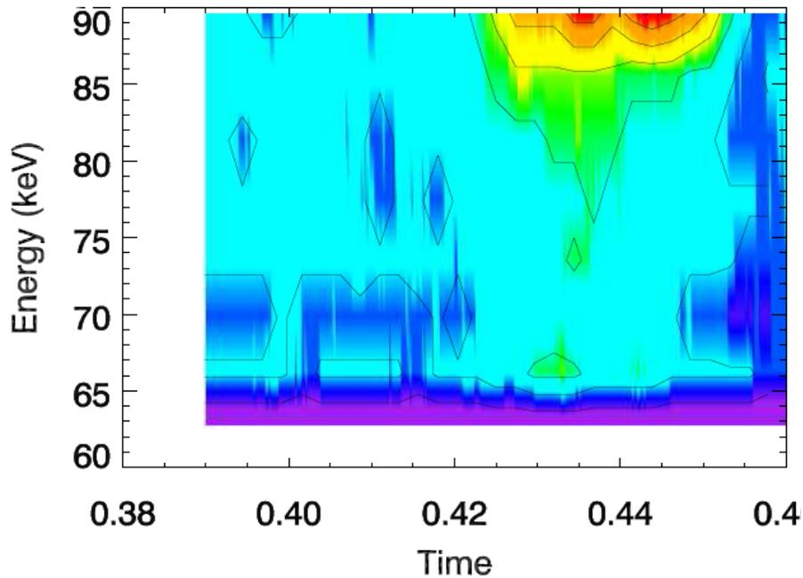
TRANSP Simulation of NPA Spectrum
