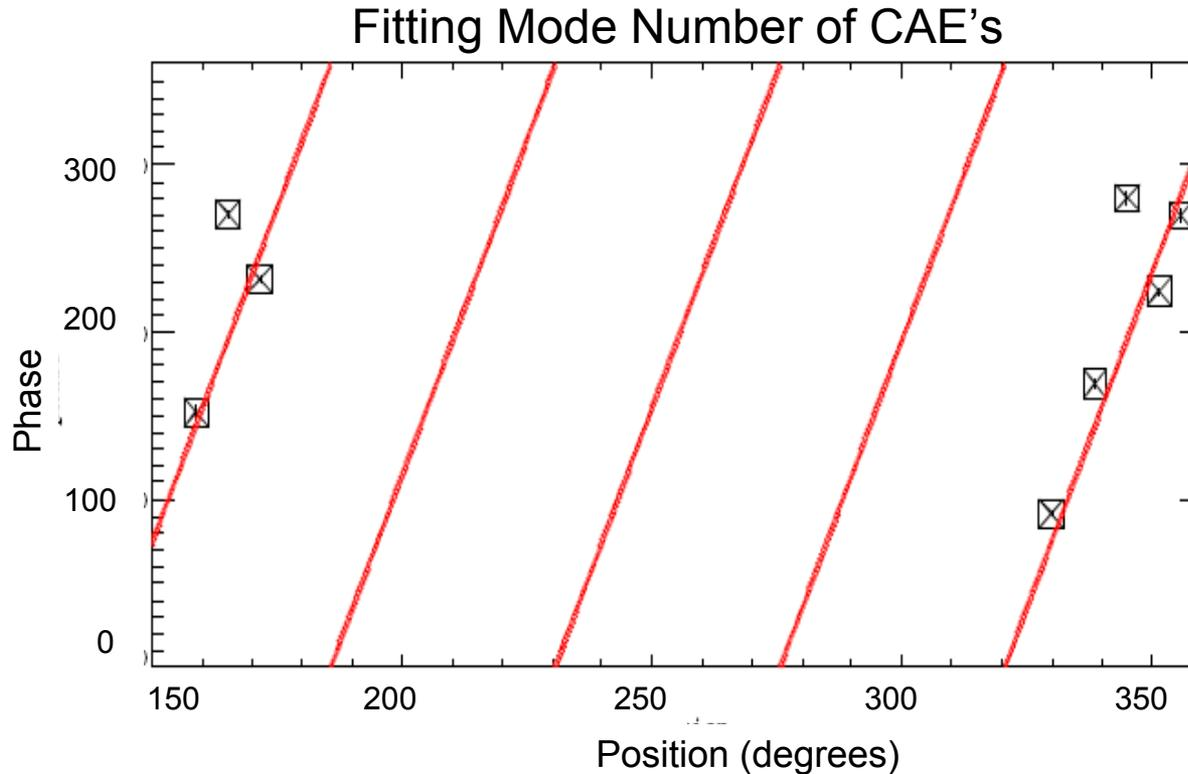
High frequency modes normally have toroidal mode numbers in the range of 7-9. Each mode must be analyzed specifically to determine mode numbers.
