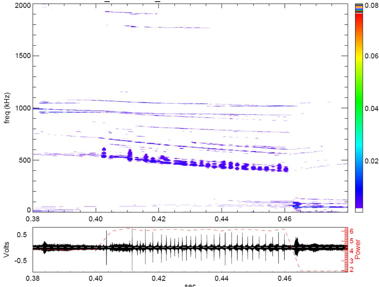
When the 3<sup>rd</sup> source turns on, some mid frequency MHD 'bursting' activity occurs. The modes are driven by fast ions, but it is not clear why these modes are bursting.
