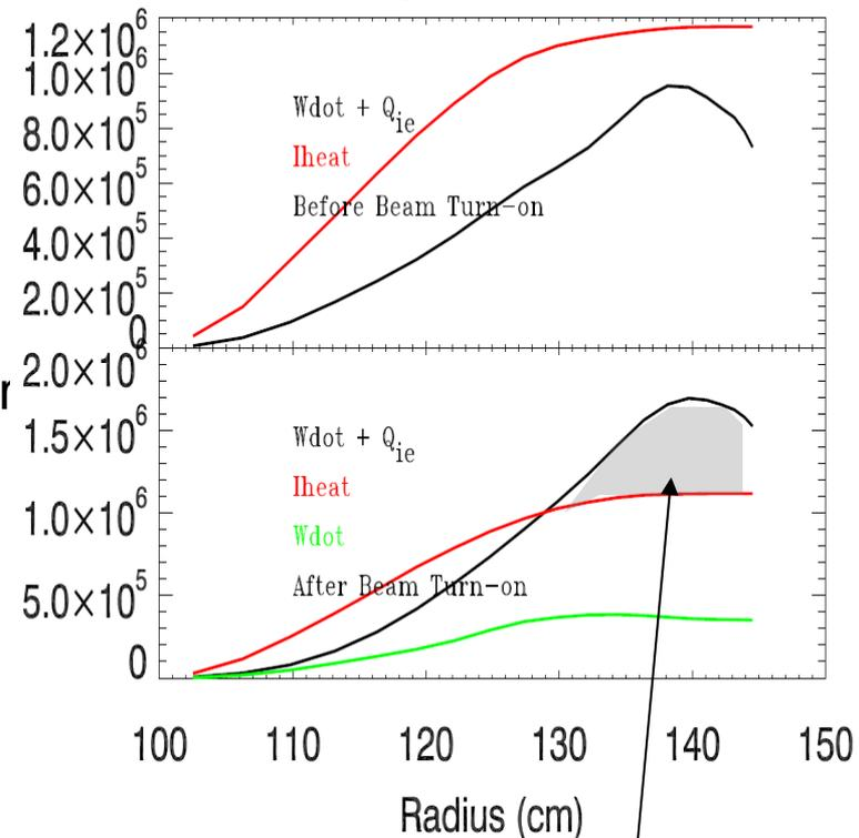
Before the 3<sup>rd</sup> beam turns on, the heating power is above the loss. After the 3<sup>rd</sup> beam turns on, the loss dominates the heating, implying an excess heating mechanism
