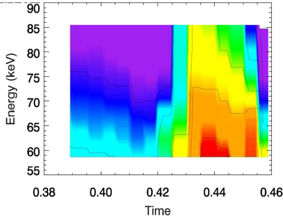
TRANSP simulations show the expected slowing down spectrum. The beam turn-on is clearly visible, and the lower energies fill up with 30 ms of the beam turn on. This fits well with classical slowing-down theory.
