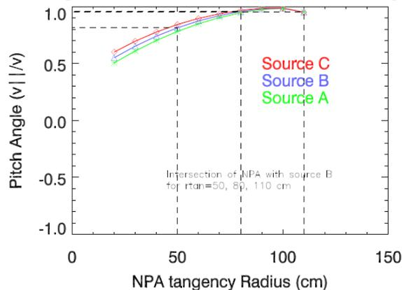
When the TRANSP calculations of NPA signals are corrected the large Larmour radius on NSTX, it is shown that the spatial intersection of the NPA with the exiting neutralized beam ions is much narrower than previously thought
