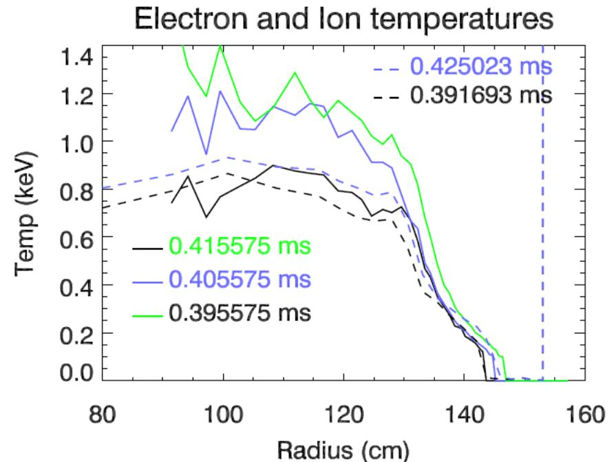
Electron (dashed) and ion (solid) temperatures. The ion temperature rises quickly after the beam turn on at 400 ms. The electron temperature rises only slightly.
