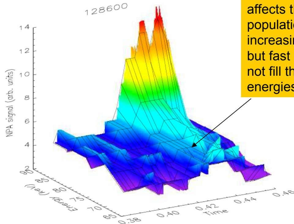
Beam turn on affects the neutral population, increasing all signal, but fast particles do not fill the lower energies
