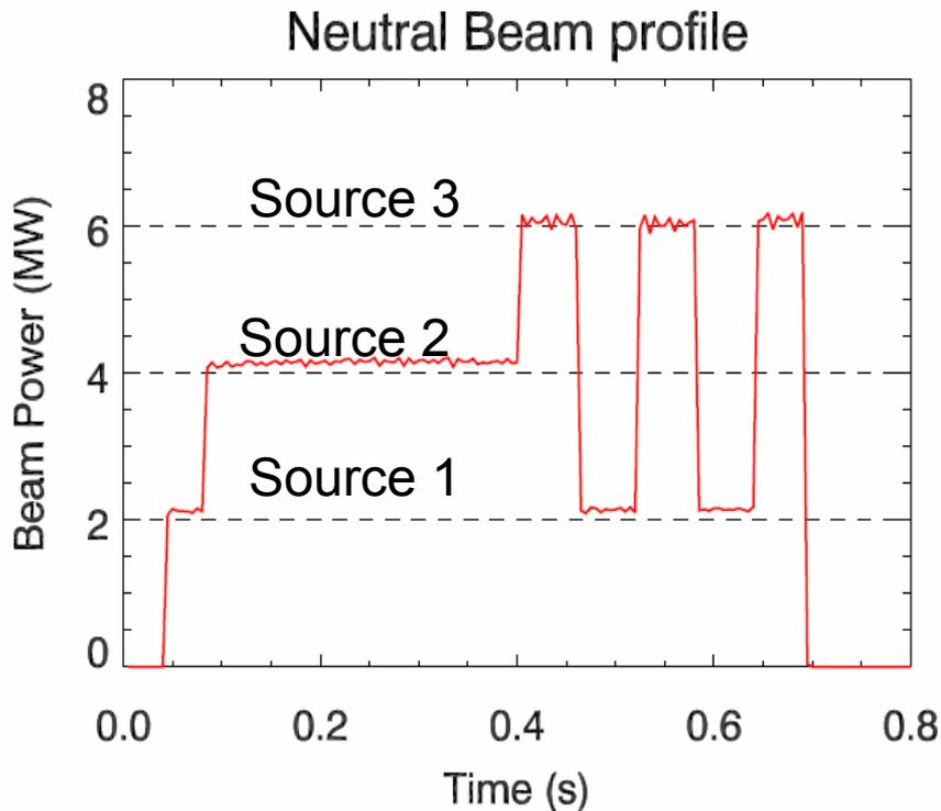
The Neutral Beam profile. The Third beam turns on at 400 ms. This coincides with the MHD free period.
