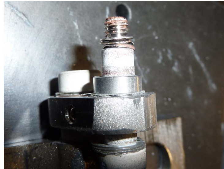
LLD plate support structural damage
