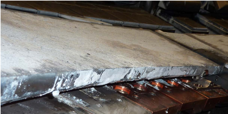
Arc damage in LLD heating tubes
