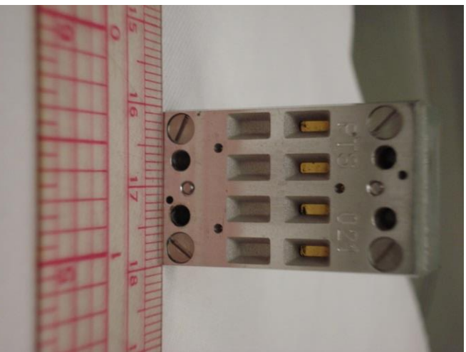
4-channel resistive bolometer from IPT-Albrecht
