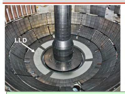
LLD plate covered with lithium Significant over-flow evident consistent with evaporating 2 x fill capacity
