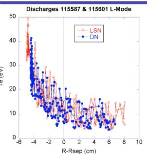
L-Mode LSN and DN, 800 kA, 1.2 MW NBI, 2 MW Pin, ne~2.2  $10^{13}$  cm<sup>-3</sup>
