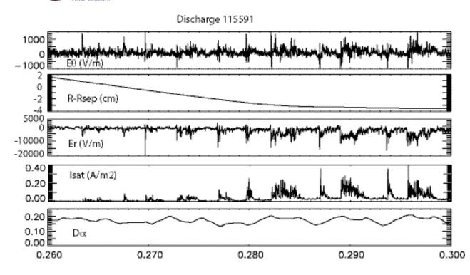
Probes measure ELM plasma parameters with high (1 MS/s) time resolution.
