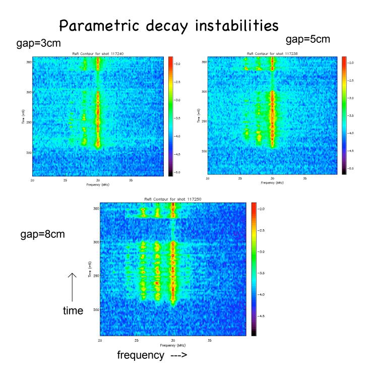
Power in instabilities increases with gap. Perhaps due to the fact that the bigger is the Gap, the higher could be the voltage on the antenna.
