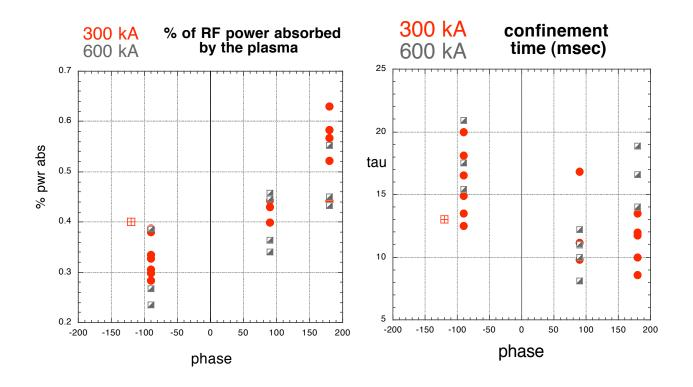
As mentioned, co-CD (-90°) has lower heating efficiency in spite of having higher confinement time.
