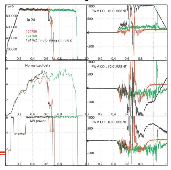
Possible convergency of feedback currents and higher beta (up to 0.6 s) suggest procedure was working
