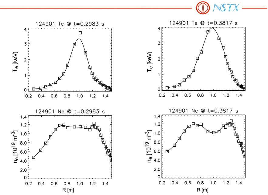
Drop in fluctuations coincides with formation of a density hole in plasma center
