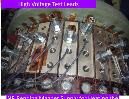
NB Bending Magnet Supply for Heating the OH Coil
