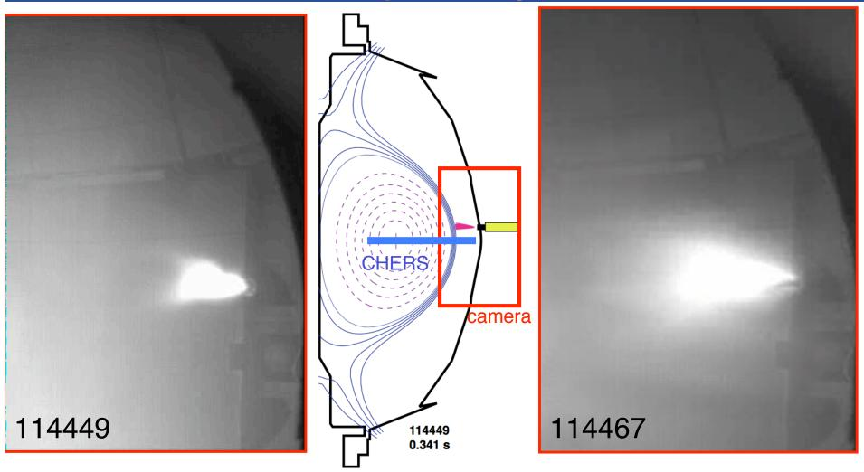
Injection in the end of discharge into a 25 cm SOL with  $T_e < 5 \text{ eV}$ ,  $n_e < 5 \times 10^{12} \text{ cm}^{-3}$  plasma
