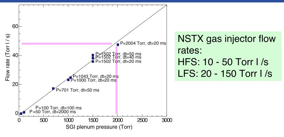
• Flow rate (Torr I / s):  $\Gamma = V_{NSTX} \Delta P / \Delta t$
