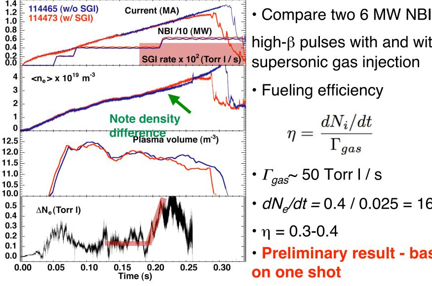
high- $\beta$  pulses with and without supersonic gas injection
