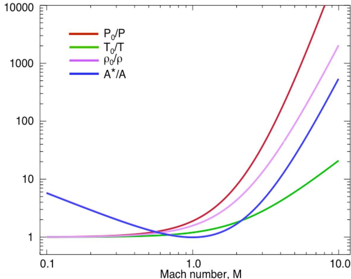
Isentropic ratios determine supersonic gas jet properties  $P$ ,  $T$ ,  $\rho$  as a function of Mach number in reference to reservoir parameters  $P_0$ ,  $T_0$ ,  $\rho_0$
