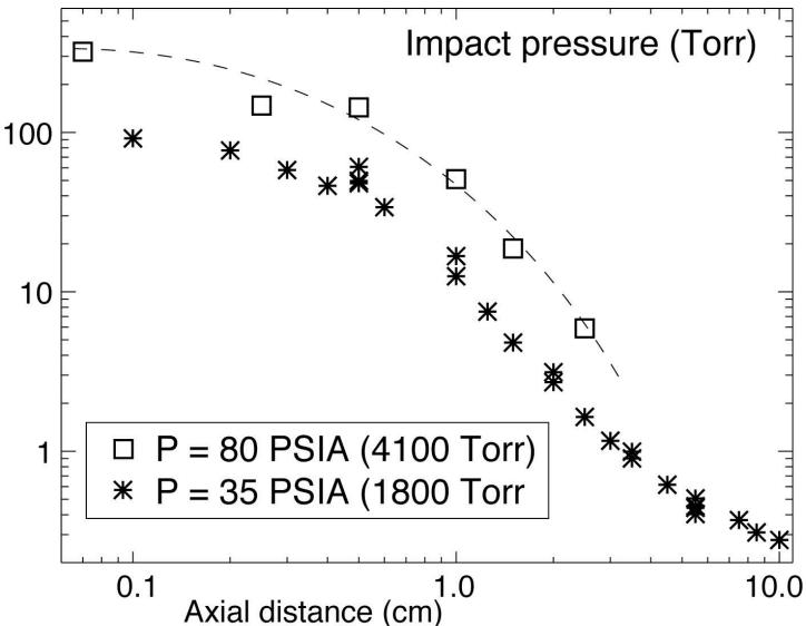
• Measurements done in deuterium by translating pressure probe axially
