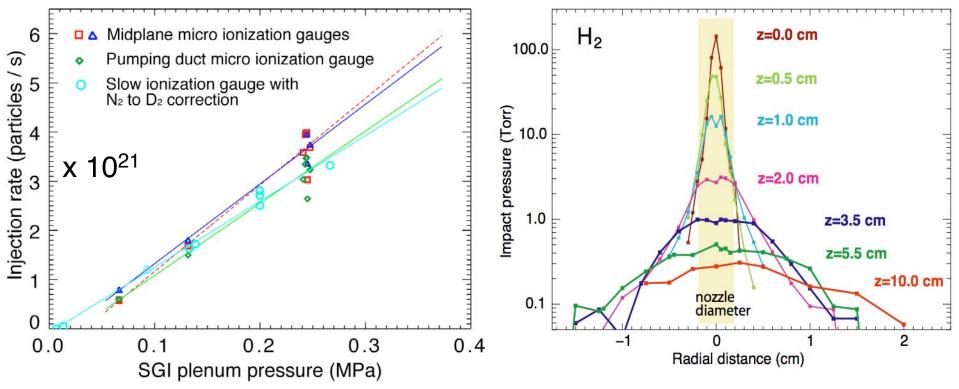
• NSTX SGI is operated at flow rates 20-125 Torr I /s (1.5 - 8.75  $\times$  10<sup>21</sup> s<sup>-1</sup>)
