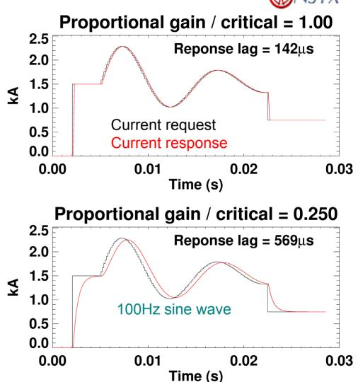
Gain parameters of SPA internal controller would need to be tuned w.r.t. actual load to minimize phase lag for optimal RWM control
