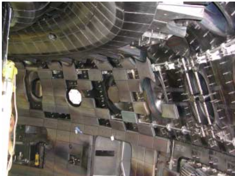
Figure 2 – DIID Internal Coils
