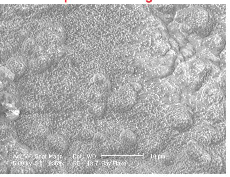
• Photo using 10 kV SEM at 10  $\mu m$  resolution of Bay F Upper Divertor thick flake obtained from the local lithium HeGDC buildup near the output of LITER showing finer Li nucleation during codeposition.
