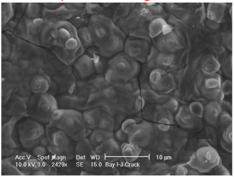
• Photo using 10 kV SEM at 10  $\mu$ m resolution of Bay I-J Midplane silicon coupon showing Li nucleation clustering.
