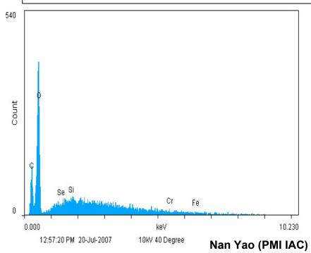
• This result is consistent with the deposition of typical plasma impurities on the Midplane Coupon and no metal output from LITER.
