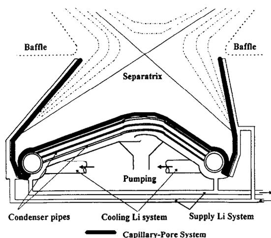
Fig. 3. LM lithium divertor with capillary-pore system design scheme.
