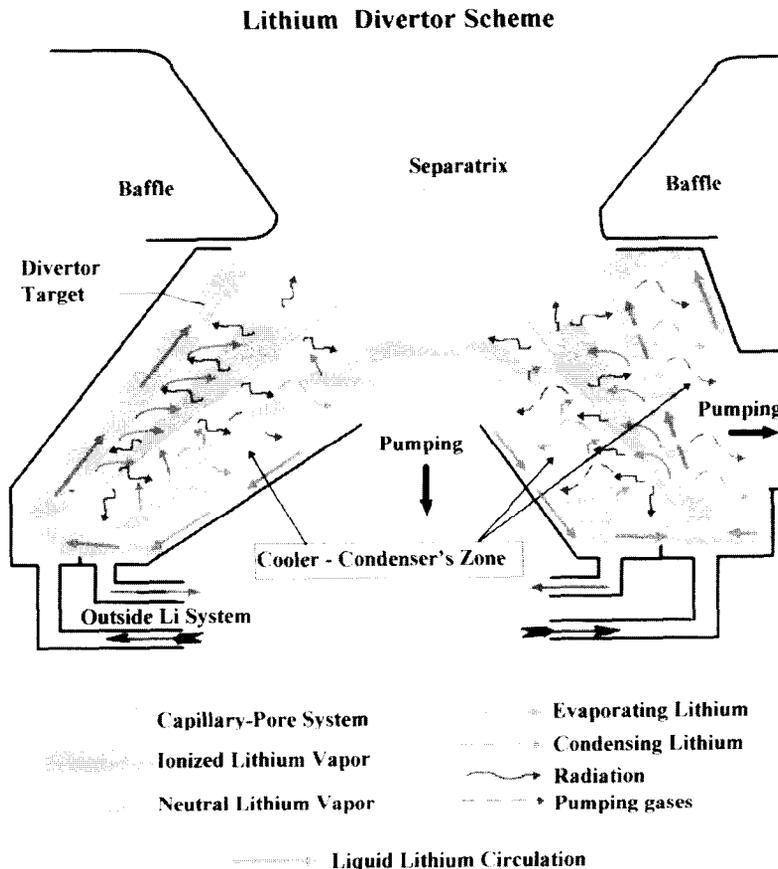
Fig. 2. The scheme of LMD energy transformation and lithium circulation.
