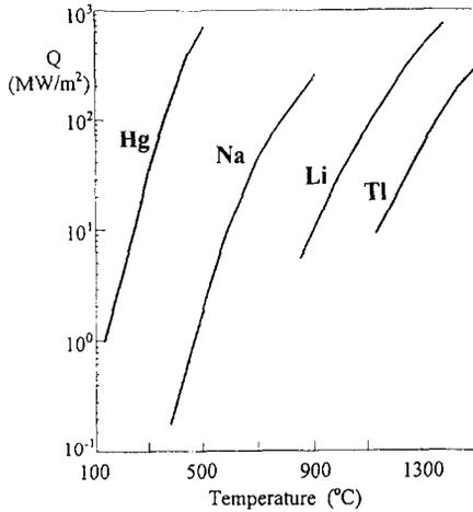
Fig. 1. Maximum thermal load released at open surface evaporation.
