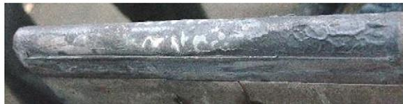
**Figure 6.** View of rail CPS Li limiter after 'cold' exposures.
