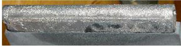
**Figure 7.** View of rail CPS Li limiter after 'hot' exposures.
