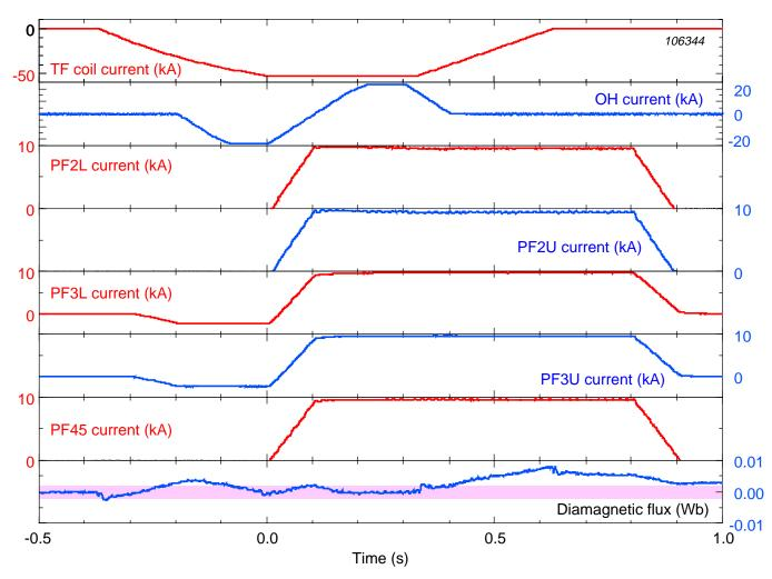
Drift during TF rampdown caused mainly by power supply imbalance
