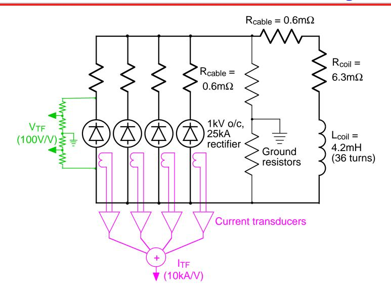
Precision DC current transducers make measurement possible
