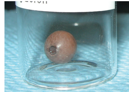
ID: 9.5 mm Wall thickness: ~120 micron Boron Mass: 0.29 gm
