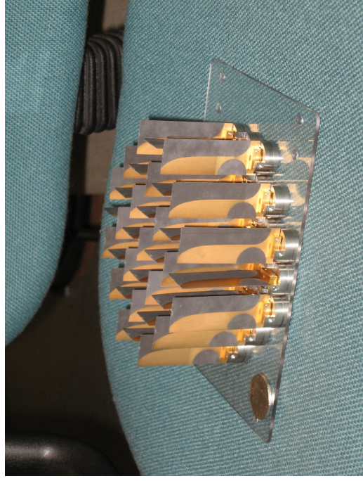
Phased array antenna
