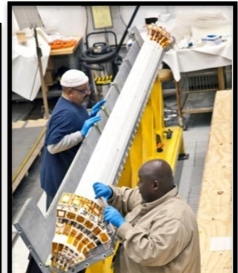
Conductors placed in a quadrant mold for VPI
