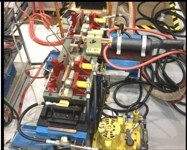
The OH in-line braze unit tested and ready for use
