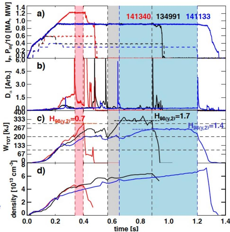
*Density rise due to carbon impurity accumulations*
