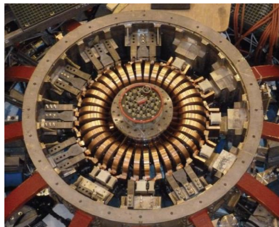
Figure 12. Upper TF flex bus installed on NSTX-U.
