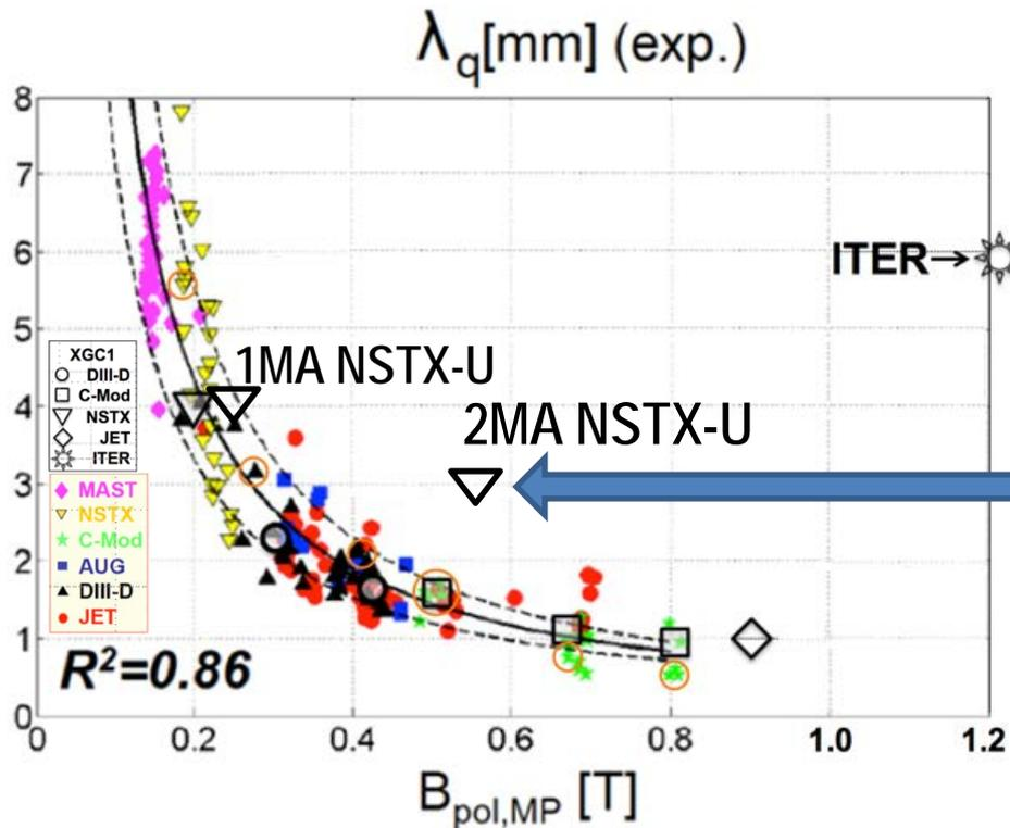
XGC1 simulations predict turbulence will widen edge heat flux in ITER
