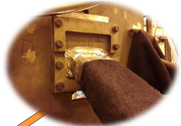
Upper Aluminum Block External Reinforcements
