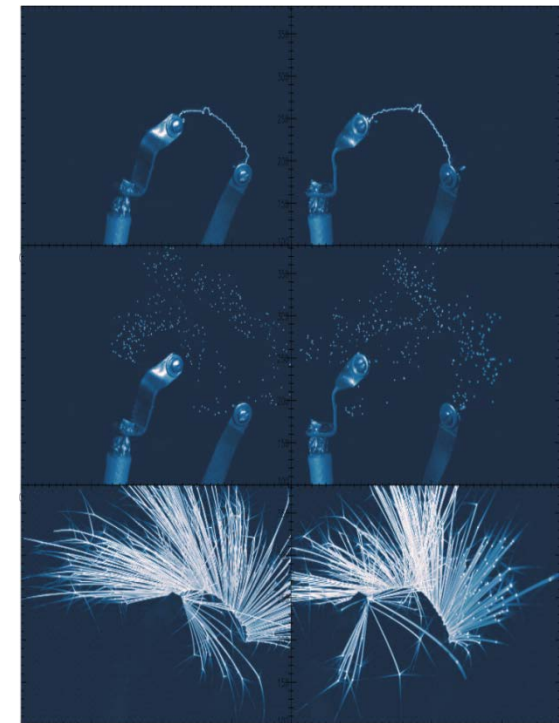
New 4D particle tracking demonstrated using an exploding-wire high-temperature microparticle source
