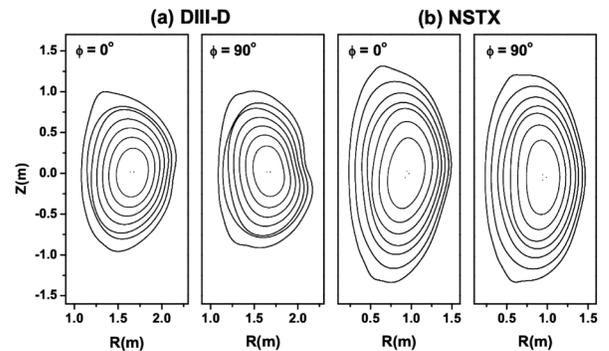
FIG. 2. The perturbed flux surfaces of (a) DIII-D and (b) NSTX target plasmas by each dominant  $n = 1$  intrinsic error field. The amplitude of the perturbation for each figure is 15 times greater than the perturbation in each machine.
