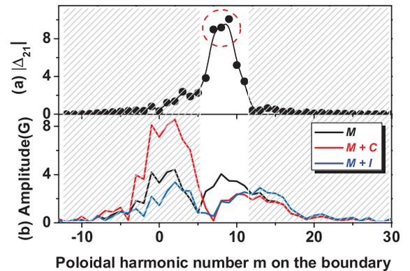
FIG. 5 (color). (a) The poloidal harmonic coupling spectrum for  $|\Delta_{21}|$  and (b) the Fourier components of the external error field on the plasma boundary in DIII-D for machine intrinsic ( $M$ ) and two optimized fields, ( $M + C$ ) and ( $M + I$ ). The dotted circle in (a) shows the most important harmonics of the external field.
