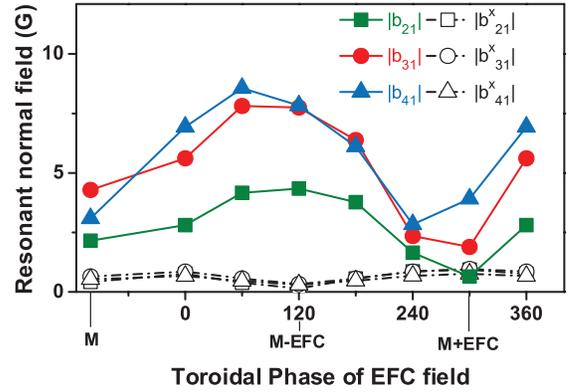
FIG. 4 (color). The variation of total  $|b_{m1}|$  and external  $|b_{m1}^x|$ ,  $m = 1, 2, 3$ , resonant fields versus the toroidal phase of the EFC-correcting field. Note opposite predictions and good consistency with the total resonant fields for the best and worst phases.
