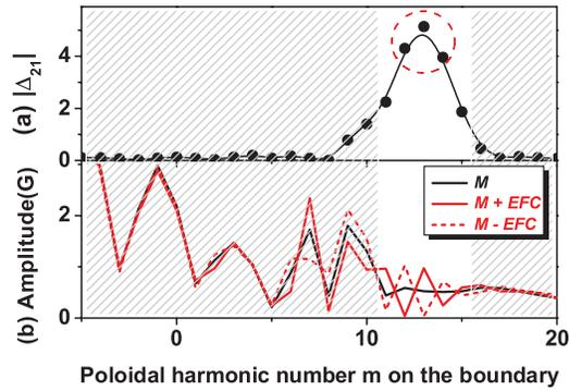
FIG. 6 (color). (a) The poloidal harmonic coupling spectrum for  $|\Delta_{21}|$  and (b) the Fourier components of the external error field on the plasma boundary in NSTX for machine intrinsic ( $M$ ), the best ( $M + EFC$ ), and the worst ( $M - EFC$ ) fields. The dotted circle in (a) shows the most important harmonics of the external field.
