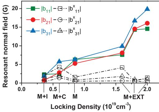
FIG. 3 (color). The total  $|b_{m1}|$  and external  $|b_{m1}^x|$ ,  $m = 1, 2, 3$  resonant fields versus locking densities in each finalized case: machine intrinsic field ( $M$ ),  $C$  coil ( $M + C$ ), and  $I$  coil ( $M + I$ ) optimized fields, and several external field correcting ( $M + \text{EFC}$ ) fields. Note the linear correlations and the amplifications in the total resonant fields compared with the external resonant fields.
