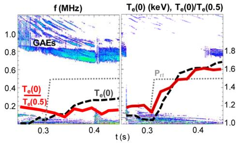
FIG. 4 (color online). Correlation between level of GAE activity and the evolution of the central  $T_e$  in rf heated NSTX  $H$  modes sustained by continuous 2 MW beam injection. The level of peaking in the central profile is characterized by the ratio  $T_e(r/a = 0)/T_e(r/a = 0.5)$ .
