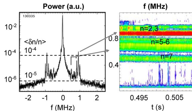
FIG. 5 (color online). Power spectrum of line integrated density fluctuations due to GAE activity in 6 MW, 1 MA, 0.45 T NSTX  $H$  mode, measured with the high- $k$  microwave scattering diagnostic in interferometric mode at  $t \sim 0.5$  s [18]. Also shown on the right is the magnetic fluctuations spectrum using a 0.05 ms time window for analysis.
