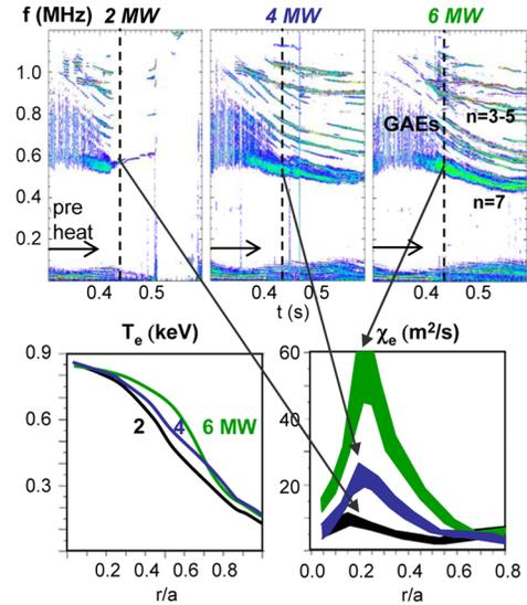
FIG. 3 (color online). Correlation between GAE activity,  $T_e$  flattening, and central  $\chi_e$  increase in NSTX  $H$  modes heated by 2, 4, and 6 MW neutral beam, at  $t \sim 0.44$  s. Within the uncertainties, the  $q$ ,  $n_e$ , and  $\omega_{E \times B}$  profiles are the same in all discharges at the time of the transport correlation [13].
