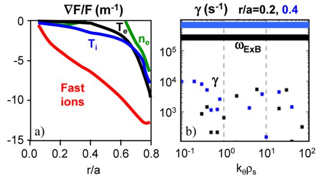
FIG. 2 (color online). (a) Thermal and density gradients in the 6 MW NSTX  $H$  mode. Also shown is the gradient in the fast ion density computed by TRANSP. (b) Linear microstability assessment of 4 MW 1 MA, 0.45 T NSTX  $H$  mode, at  $r/a = 0.2$  and  $0.4$  ( $t = 0.5$  s). The most unstable growth rates are shown as a function of  $k_\theta \rho_s$ . Also shown as bands is the range of  $\mathbf{E} \times \mathbf{B}$  shearing rates computed by TRANSP [10].
