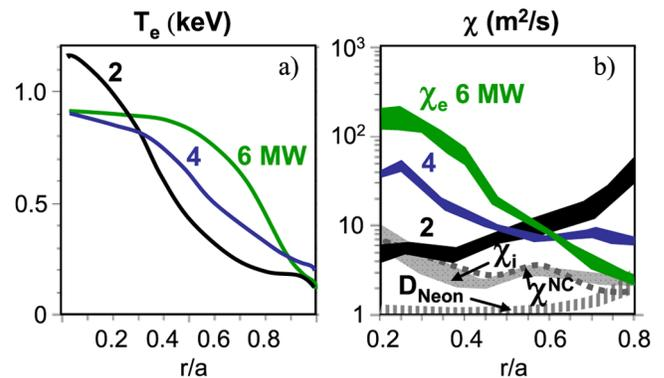
FIG. 1 (color online). (a)  $T_e$  profiles in 2, 4, and 6 MW NSTX  $H$  modes at  $t \sim 0.4$  s. The measurement uncertainty is around 25 eV. (b) TRANSP computed  $\chi_e$  in the same plasmas. Also shown are the  $\chi_i$  and NCLASS ion thermal diffusivity for the 6 MW case and the measured neon diffusivity. The bands of values represent the 20 ms variability.
