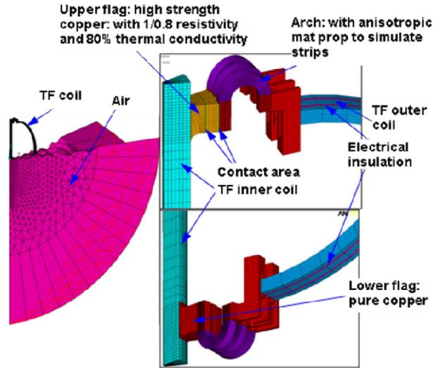
Fig. 4. Electromagnetic Model.
