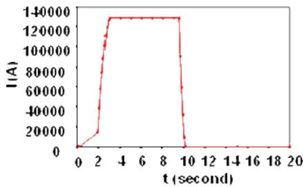
Fig. 3. NSTX TF coil current (unit: A).
