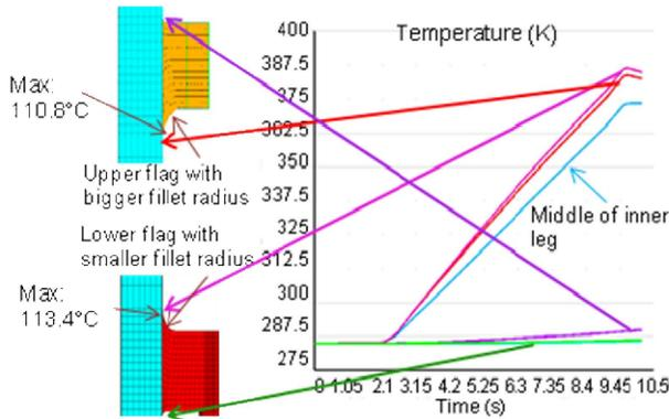
Fig. 6. Temperature rise in TF inner coil with water cooling.
