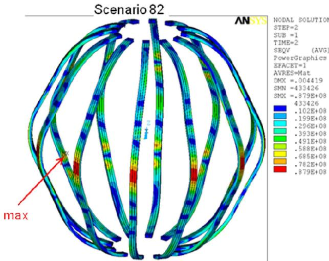
Fig. 10. Coil Von Mises stress (Pa).
