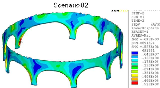
Fig. 12. Von Mises stress (Pa) of umbrella arch.
