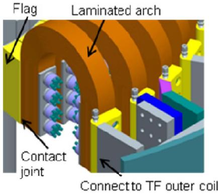
Fig. 2. Connection between TF inner and outer coils.
