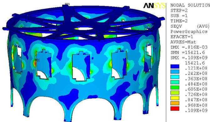
Fig. 11. Umbrella structure Von Mises stress (Pa).
