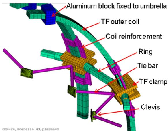
Fig. 9. Modeling of TF outer coil and TF truss.
