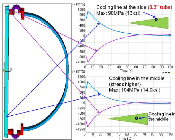
Fig. 7. History plot of stress  $S_{\theta}$  (Pa) in TF coil with water cooling.
