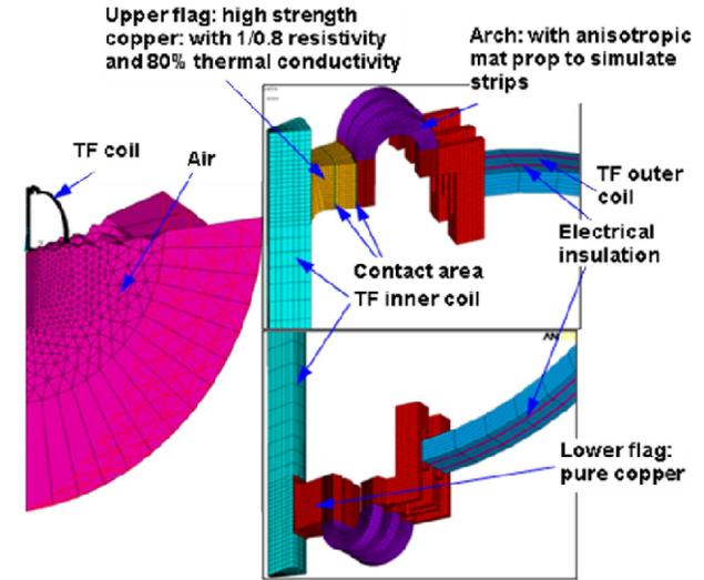
Fig. 4. Electromagnetic Model.
