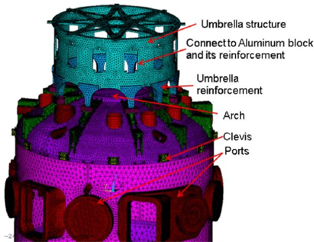
Fig. 8. Modeling of vacuum vessel.
