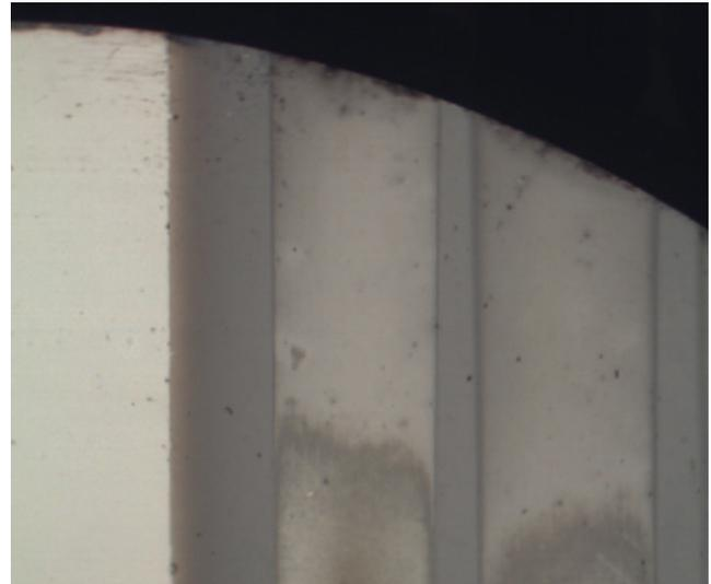
FIG. 5. Beryllium coated molybdenum mirror. The light stripe on the left is bare molybdenum; the two 1 mm wide strips on the right were treated with laser scans at  $1.6 \text{ J/cm}^2$ . Some reflectivity is restored, but not to the uncoated level.
