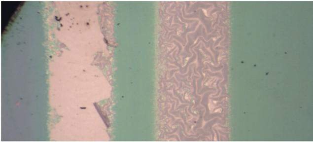
FIG. 3. Image of a molybdenum mirror coated with 422 nm of carbon after laser scans on left at  $0.9 \text{ J/cm}^2$  showing film removal and on right at  $0.7 \text{ J/cm}^2$  with film buckling. The laser track is 1.1 mm wide.
