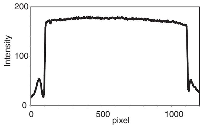
FIG. 2. Lineout of the aluminum reference mirror illustrating uniformity of illumination.
