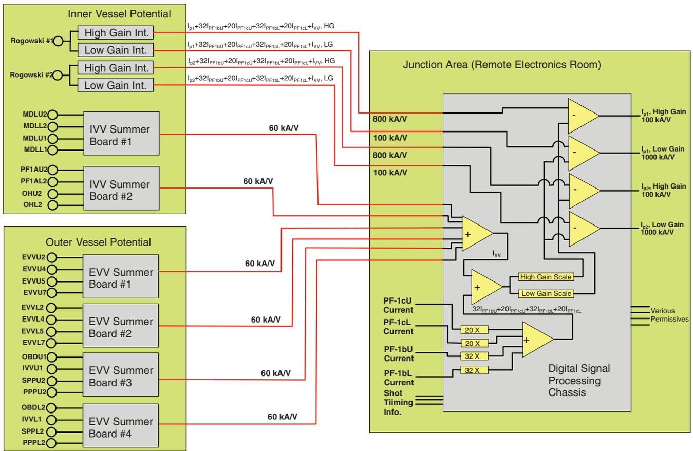
FIG. 3. Schematic of the  $I_p$  calculator for NSTX-Upgrade.
