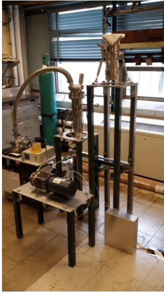
Figure MP-6: Current status of integration of the liquid-lithium test-stand. Reservoirs are shown at upper right and the liquid metal, permanent magnet pump is shown at bottom left.
