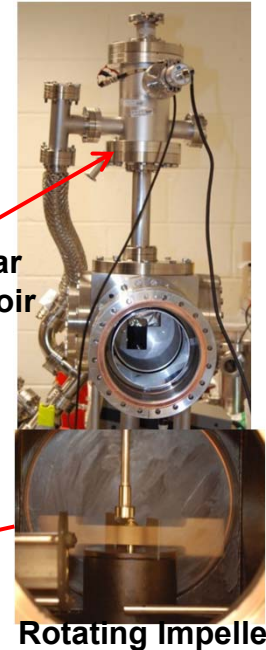
Granule injector (GI) for ELM pacing
