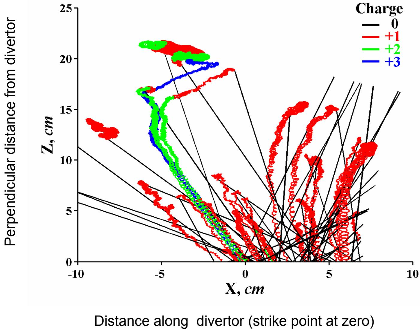
WBC Simulation of LLD sputtered lithium transport: 50 trajectories shown;
