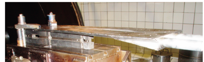
Lithium module in the process of electron beam welding
