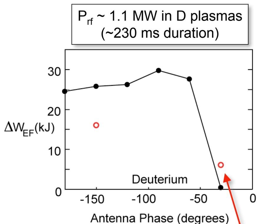
Noticeable increase in  $\Delta W_{EF}$  with  $-30^\circ$  phasing in D plasmas with Li edge conditioning, even with shorter rf duration (67 ms)
