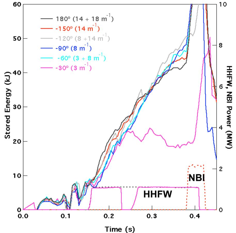
Heating efficiency drops for  $|\Delta\phi| < 60^\circ$  due to high edge density and MHD
