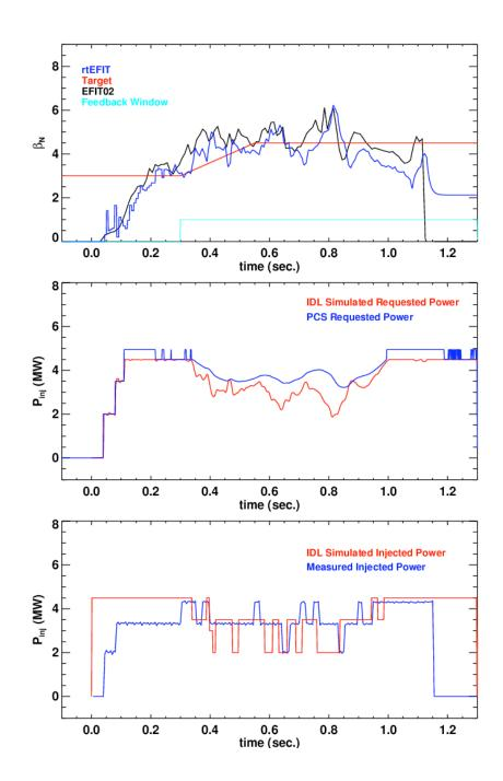
Optimal Setting May Involve a Longer Time Constant, Derivative Gain, and Small Integral Gain
