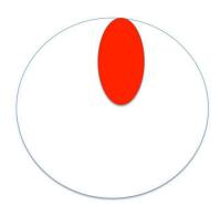
A helical distortion pushes the plasma towards the wall at some  $\varphi$  and pulls the plasma from the wall at other  $\varphi$ .
