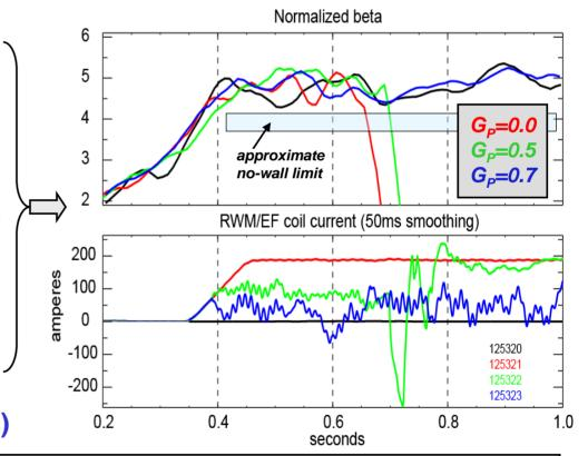
→ Use same gain/phase settings to suppress RFA from intrinsic EF **and** any unstable RWMs
