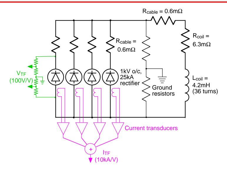
Precision DC current transducers make measurement possible
