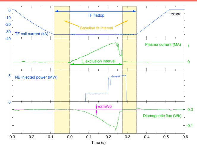
♦ Fit coefficient of resistive flux varies by about 1% with temperature of air-cooled buswork; coefficient of inductive flux varies by <0.1%
