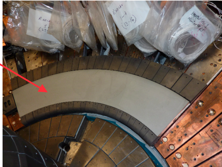
1st LLD-1 Plate Installed in NSTX
