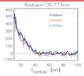
Spectra before and after burst match well at all radii
