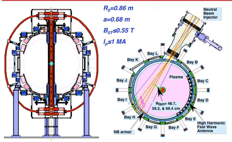
• 3 beam sources inject 80-90 kV D, ≤6 MW
