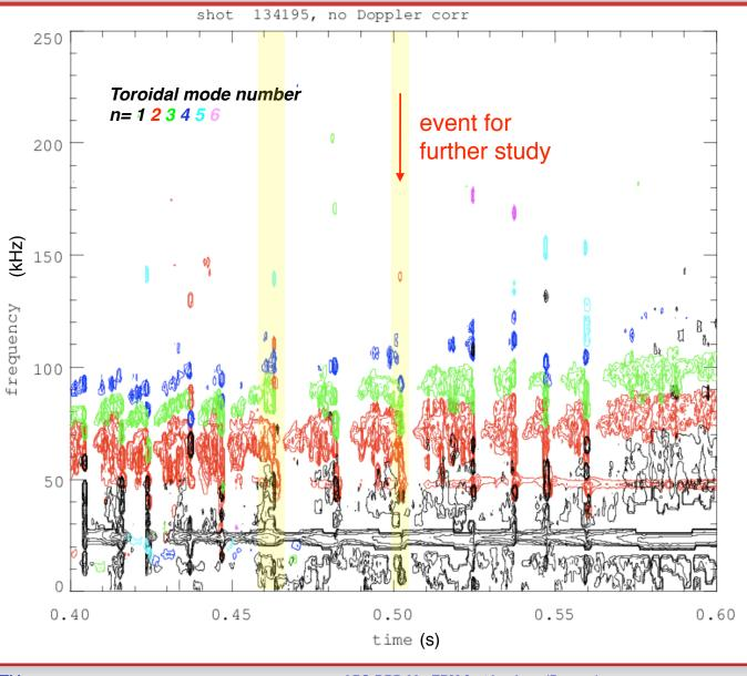
Mirnov spectrogram of numerous EPMs shown Smaller activity preceding events produces no fast ion loss
