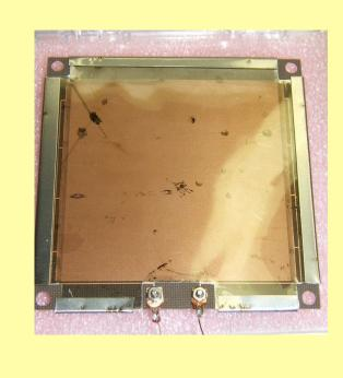
Mica cover to shield bottom grid (#2).
